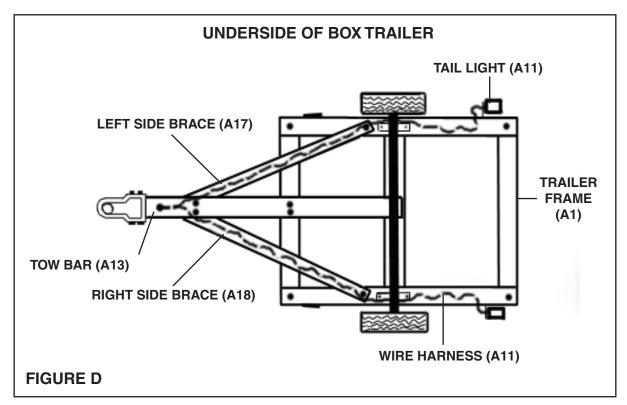
3. With assistance, carefully tip the Trailer on its side to perform this procedure. **NOTE:** It is recommended to use heavy gauge, nylon, **tie strips** (not included) to attach the wiring harnesses of the Tail Lights (A11) to the **underside** of the Frame Assembly. Once finished, carefully tip the Trailer to its upright position. **(See Figure D.)**
